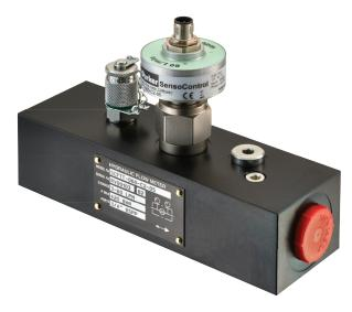
A turbine wheel is driven by the oil flow and thus set in motion. The frequencies produced are processed by a digital electronic device. The influence of disturbing flow effects is thus compensated. With the lower flow resistance  $Q_{\rm p}$ , the hydraulic circulation operates at low loss.
