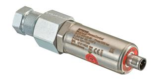
Quick response times guarantee a quick identification of disturbing pressure peaks in the hydraulic system. The robust stainless steel construction allows a variety of applications, e. g. in hydraulics, for cooling water or in compressed air systems.
