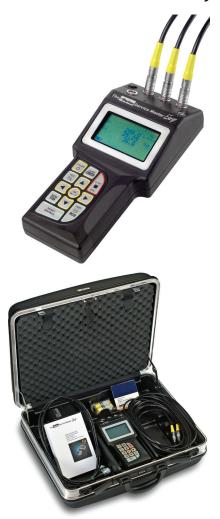
**The Parker Service Master** *Easy* is a multi-channel portable measurement instrument for the simultaneous measurement of important hydraulic units:
