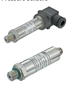
The **SCP-EX** can be configured for Zone 1 and conforms with Directive 94/9/EC. Thanks to the appropriate protective circuits, polarity reversal protection, overvoltage protection, and power dissipation limitation will be activated in the case of a fault. Its wide-reaching industrial application options are guaranteed through high accuracy and a robust and compact construction. Various pressure transducers are available thanks to its compatibility with different mechanical and electrical
